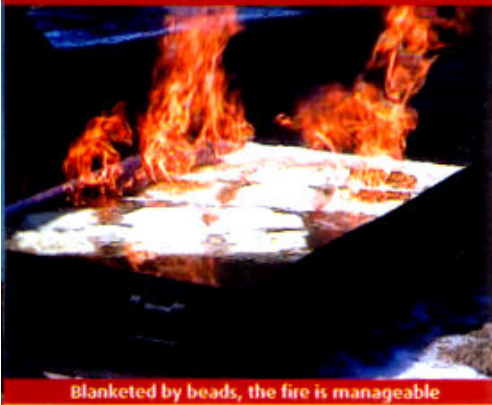
Blanketed by beads, the fire is manageable (Blanketed by Beads, the fire is manageable)
