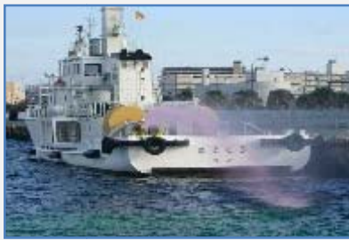
Vessel spraying the beads onto the water surface
